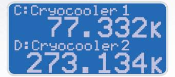
Several display formats may be selected. Up to eight temperature readings may be displayed simultaneously or two channels with input names and temperature shown in a large easy to read font. Additional screens include temperature readings along with relay and alarm status information.
