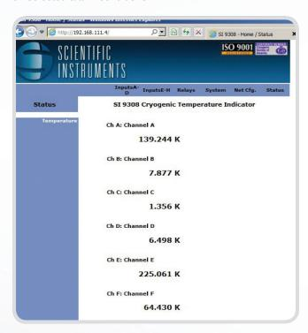
Using the Ethernet HTTP protocol, the monitor's embedded web server allows the instrument to be viewed and configured from any web browser.
